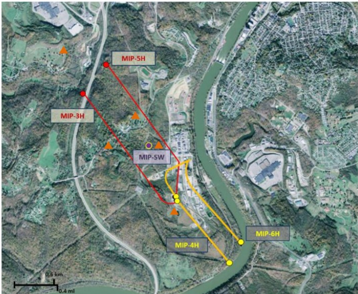
Figure 18: Marcellus Shale Energy and Environment Laboratory (MSEEL) just outside Morgantown, West Virginia, USA. The MSEEL site consists of four horizontal production wells operated by Northeast Natural Energy LLC. (MIP-3H, MIP-4H, MIP-5H, MIP-6H), two pilot holes (MIP-3 and MIP-4), a micro-seismic observation well (MIP-SW), and a grid of five surface seismometers (triangles).
