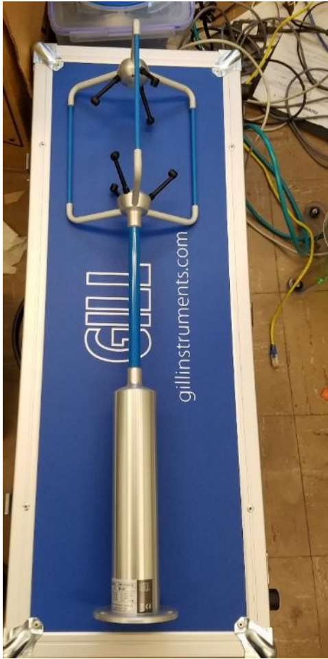
Figure 5.1. Left: new LI-7700 during DAQ interfacing and right, new Windmaster Pro.
