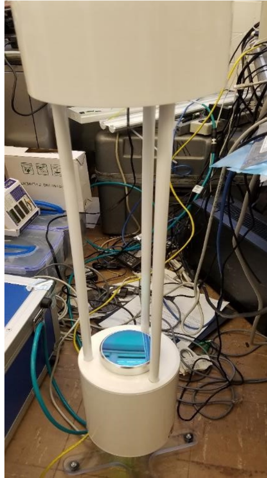
Figure 5.1. Left: new LI-7700 during DAQ interfacing and right, new Windmaster Pro.
