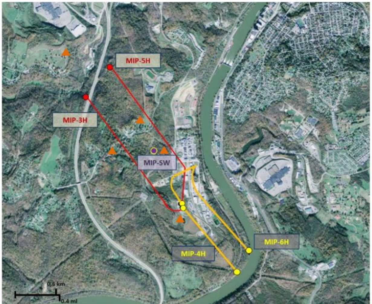
Figure 1.1: Marcellus Shale Energy and Environment Laboratory (MSEEL) just outside Morgantown, West Virginia, USA. The MSEEL site consists of four horizontal production wells operated by Northeast Natural Energy LLC. (MIP-3H, MIP-4H, MIP-5H, MIP-6H), two pilot holes (MIP-3 and MIP-4), and a micro-seismic and sampled observation well (MIP-SW), and a grid of five surface seismometer (triangles).
