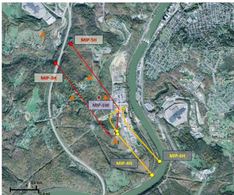
Figure 4: Marcellus Shale Energy and Environment Laboratory (MSEEL) just outside Morgantown, West Virginia, USA. The MSEEL site consists of four horizontal production wells operated by Northeast Natural Energy LLC. (MIP-3H, MIP-4H, MIP-5H, MIP-6H), two pilot holes (MIP-3 and MIP-4), and a micro-seismic and sampled observation well (MIP-SW), and a grid of five surface seismometer (triangles).
