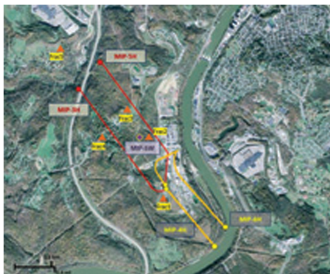
Figure 1. The MSEEL site just outside Morgantown, West Virginia, USA. The MSEEL site consists of four horizontal production wells operated by Northeast Natural Energy LLC (MIP-3H, MIP-4H, MIP-5H, and MIP-6H), two pilot holes (MIP-3 and MIP-4), a microseismic observation well (MIP-SW), and a grid of five surface seismometers (triangles). FRAC3 and FRAC4 were working intermittently during hydraulic fracturing due to a limited power supply. The location of the studied stage 10 is also shown on well MIP-3H.
