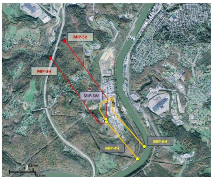
Figure 1—MSEEL outside Morgantown, West Virginia, USA. The MSEEL site consists of four horizontal production wells, MIP-3H, MIP-4H, MIP-5H, MIP-6H; two pilot holes, MIP-3 and MIP-4; and a microseismic and sampled observation well, MIP-SW (Ghahfarokhi et al. 2018).
