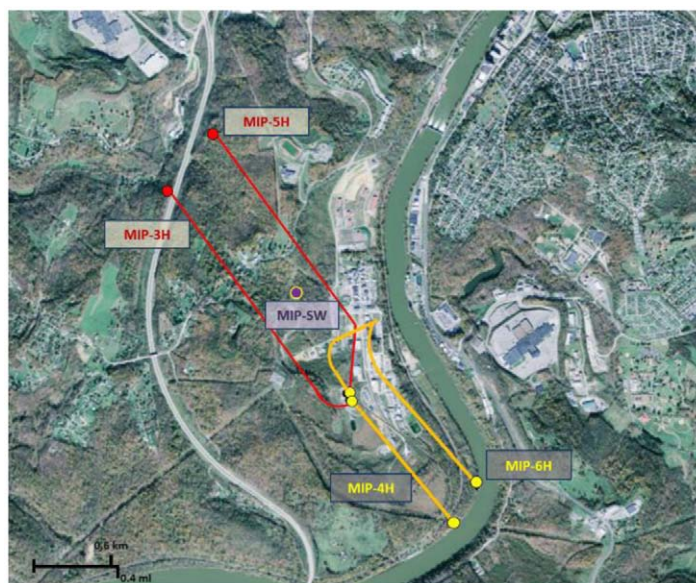
Figure 1—MSEEL outside Morgantown, West Virginia, USA. The MSEEL site consists of four horizontal production wells, MIP-3H, MIP-4H, MIP-5H, MIP-6H; two pilot holes, MIP-3 and MIP-4; and a microseismic and sampled observation well, MIP-SW (Ghahfarokhi et al. 2018).
