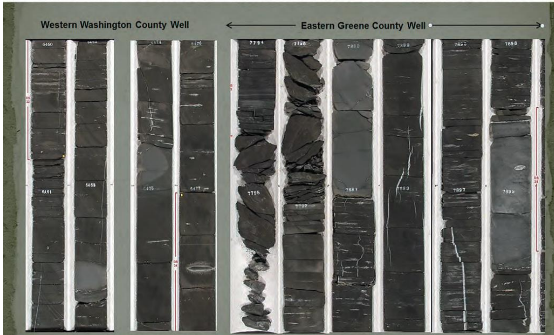
The number and width of vertical calcite filled fractures increases significantly from the Western Washington County cores the eastern Greene County cores.
