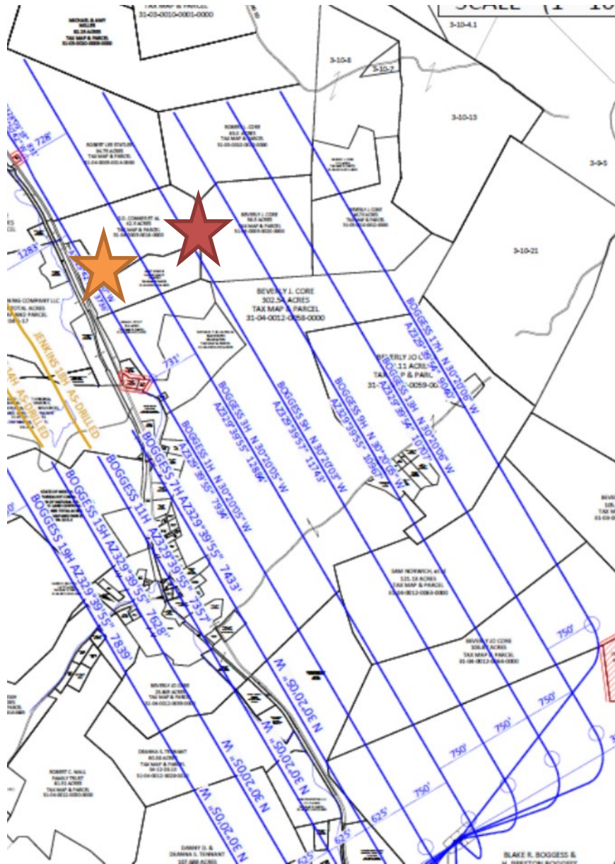
Figure 0.1: Boggess Pad with new generation permanent fiber in the central well (Boggess 5H, red star)) and deployable fiber in adjoining wells skipping one (orange stars). We were able to monitor in near-real time fracture stimulation in the central 3 wells (3H, 5H and 9H). A vertical pilot was drilled, cored and logged. We continue to collect DTS data from the 5H.
