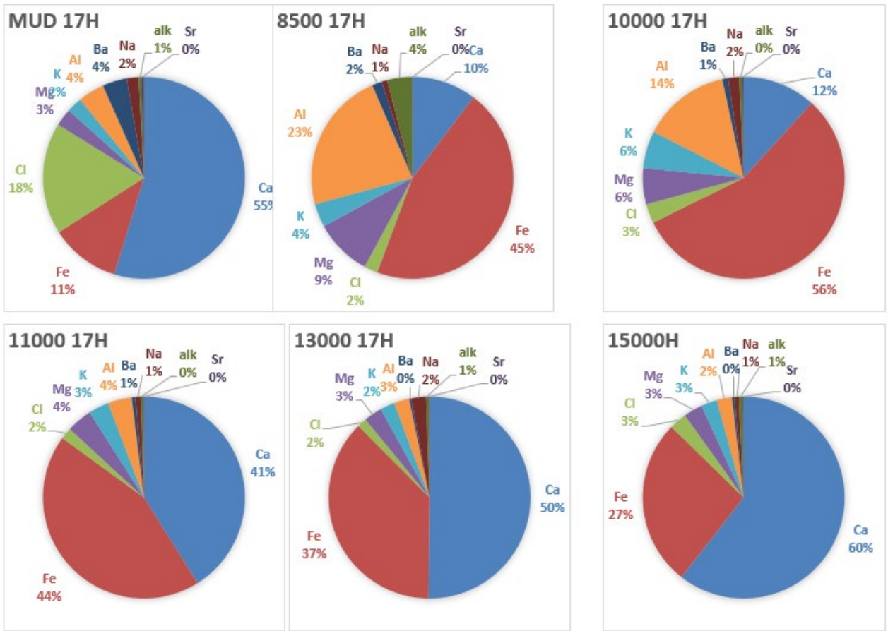
Figure 4.17. Anions/cations of drilling mud and cuttings solids from 17H.
