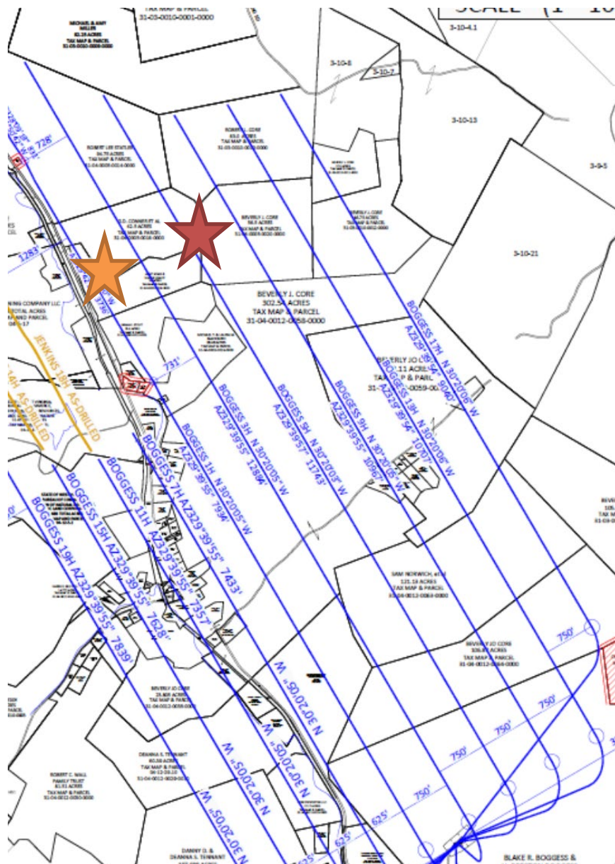
Figure 0.1: Boggress Pad with new generation permanent fiber in the central well (Boggress 5H, red star) and deployable fiber in adjoining wells skipping one (orange stars). We were able to monitor in near-real time fracture stimulation in the central 3 wells (3H, 5H and 9H). A vertical pilot was drilled, cored and logged. We continue to collect DTS data from the 5H.
