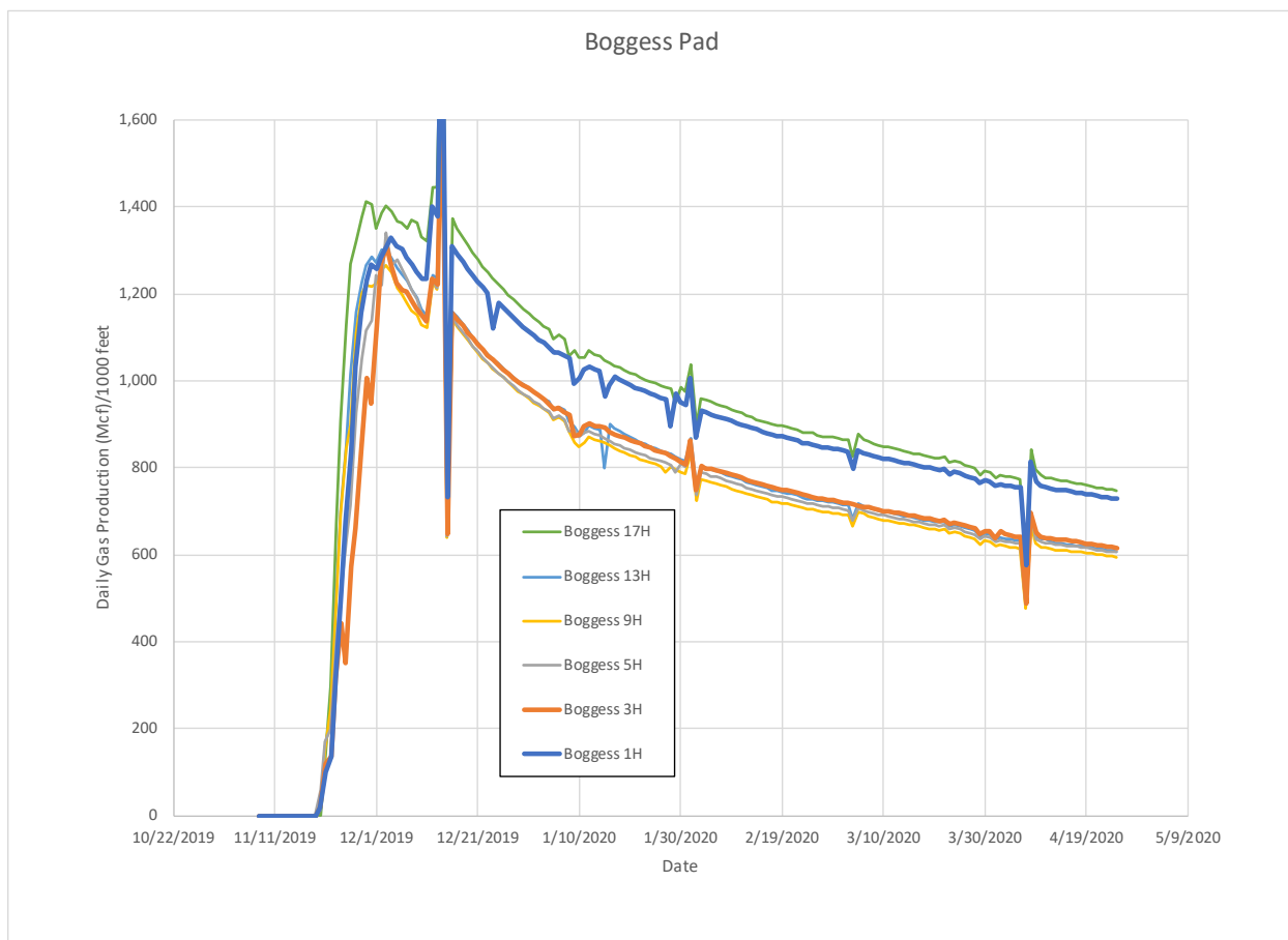
Figure 1.3: Initial daily production from the Boggess Pad normalized for Mcf per 1000’ of completed lateral. The wells engineered using the MSEEL software are highlighted with thicker lines (1H and 3H). As you can see outside wells (1H and 17H) perform better than interior wells due to reduced competition. Also wells engineered using the MSEEL approach got off to a slower start but have narrowed the gap in daily production and in the case of the 3H are producing more than any other interior well. In the case of the 1H compared to 17H the gap is narrowing. In the 17H, more sand was used per stage and we need to adjust for sand per foot. The production is early, and the picture could very easily change.
