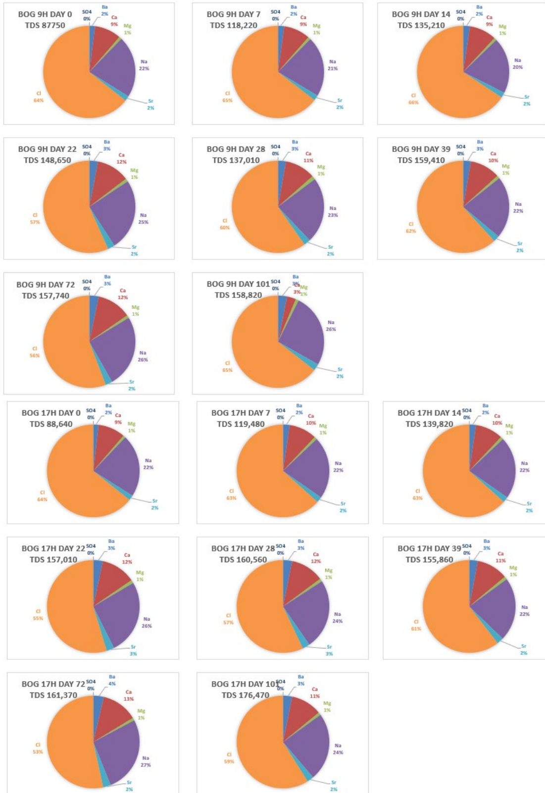
Figure 4.17. Major ion concentrations in produced water from wells BOGESS 9H and 17H.
