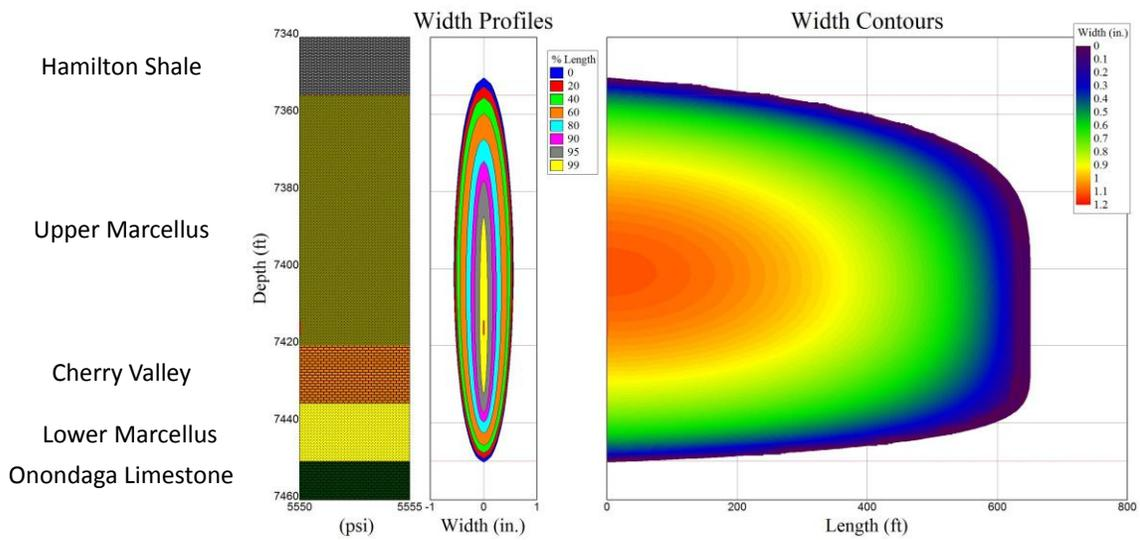
**Figure 4.b.7: Fracture Geometry for Stage 3 - MIP 3H**
