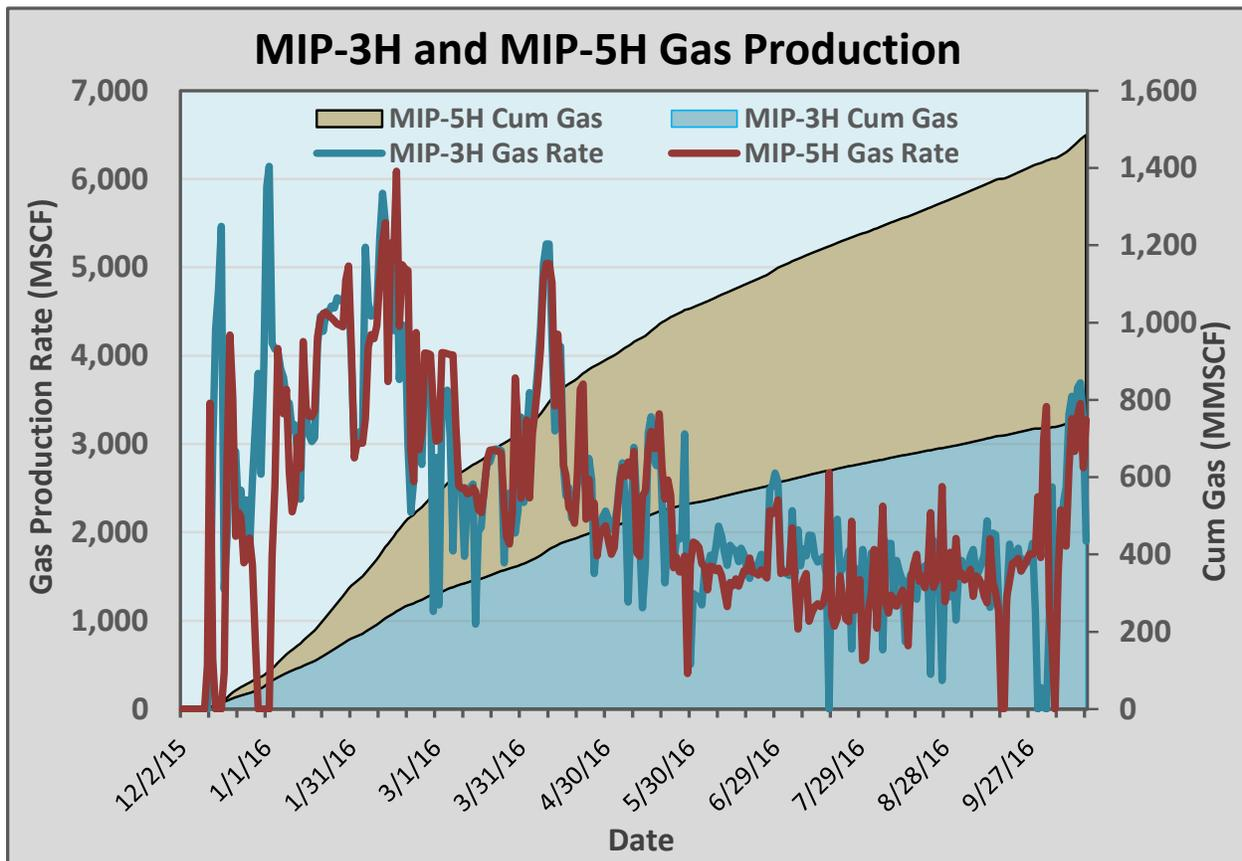
**Figure 2.1 Daily and cumulative gas production from the MIP 3H and MIP 5H at the MSEEL site. Gas production was curtailed beginning in May 2016 due to weak demand. Production has begun to increase at the end of September 2016.**
